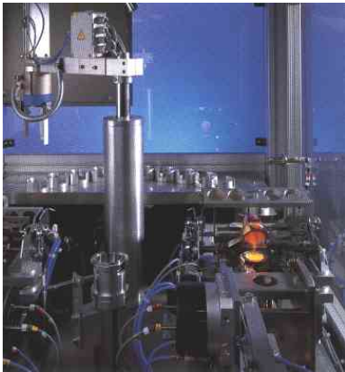
The pyrometer located above the burner monitors the fusion temperature during the fusion process, ensuring that the temperature characteristic is adjusted to the sample quality.
