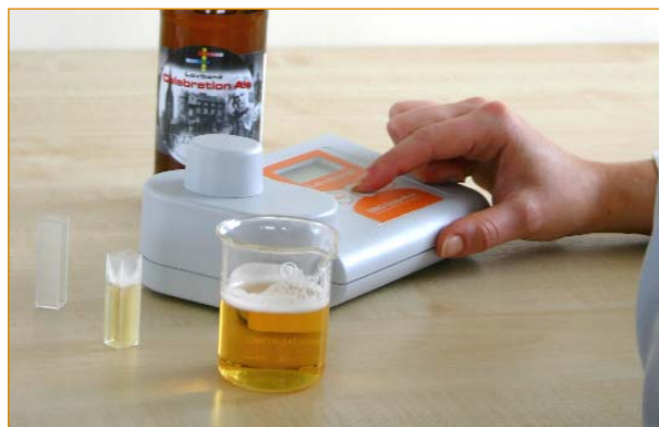
Switch the ColorPod on and ZERO using a cell filled with distilled water.
