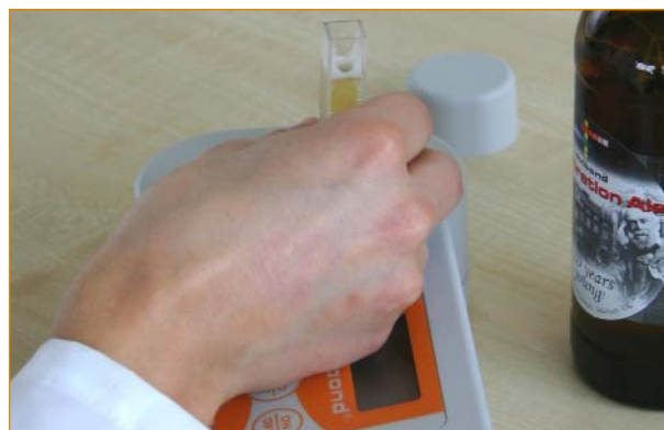
Insert the sample-filled cell and press TEST. Results will be shown in EBC units.
