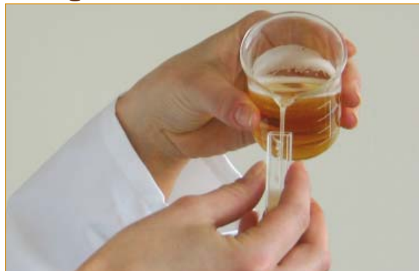
Fill a cell with the sample to be tested. Ensure the outside of the cell is clean and dry. (Wipe gently with a clean tissue)
